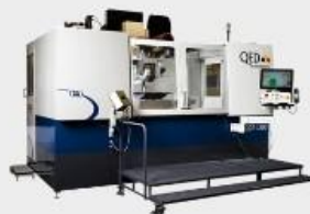
Magnetorheological Finishing (<math>\varnothing</math> 1200 mm)
